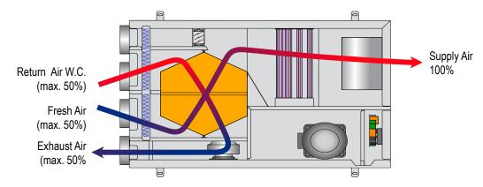
Whit this selected mode, the unit renews the ambient air with the outside through the heat exchanger of high efficiency.
