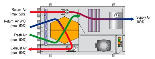
GHE 26 units can operate with a flow rate of outdoor air from 80 to 130 m³/h (140 to 260 m³/h for the model GHE 51), to ensure sufficient supply air changes in the room having a variable volume by 260 m³ (0.5 vol/h) to 460 m³ (0.3 vol/h), in compliance with regional and national regulations. The air flow
