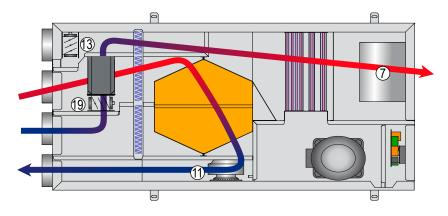
The compressor is off, the water coil is not powered (3-way valve closed), the recirculation damper (13) is closed, the damper by-pass of the recuperator (19) is open.
